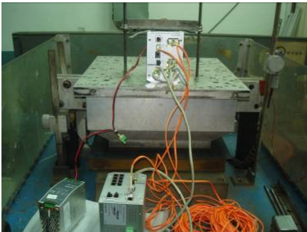
Fig. 9: Switching Hub (JetNet 5012G) Shock Test in \pm Z Axis -2
