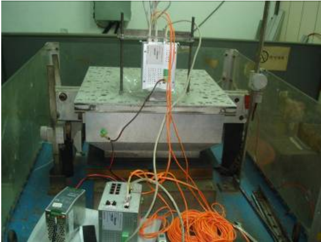
Fig. 7: Switching Hub (JetNet 5012G) Shock Test in \pm X Axis -1
