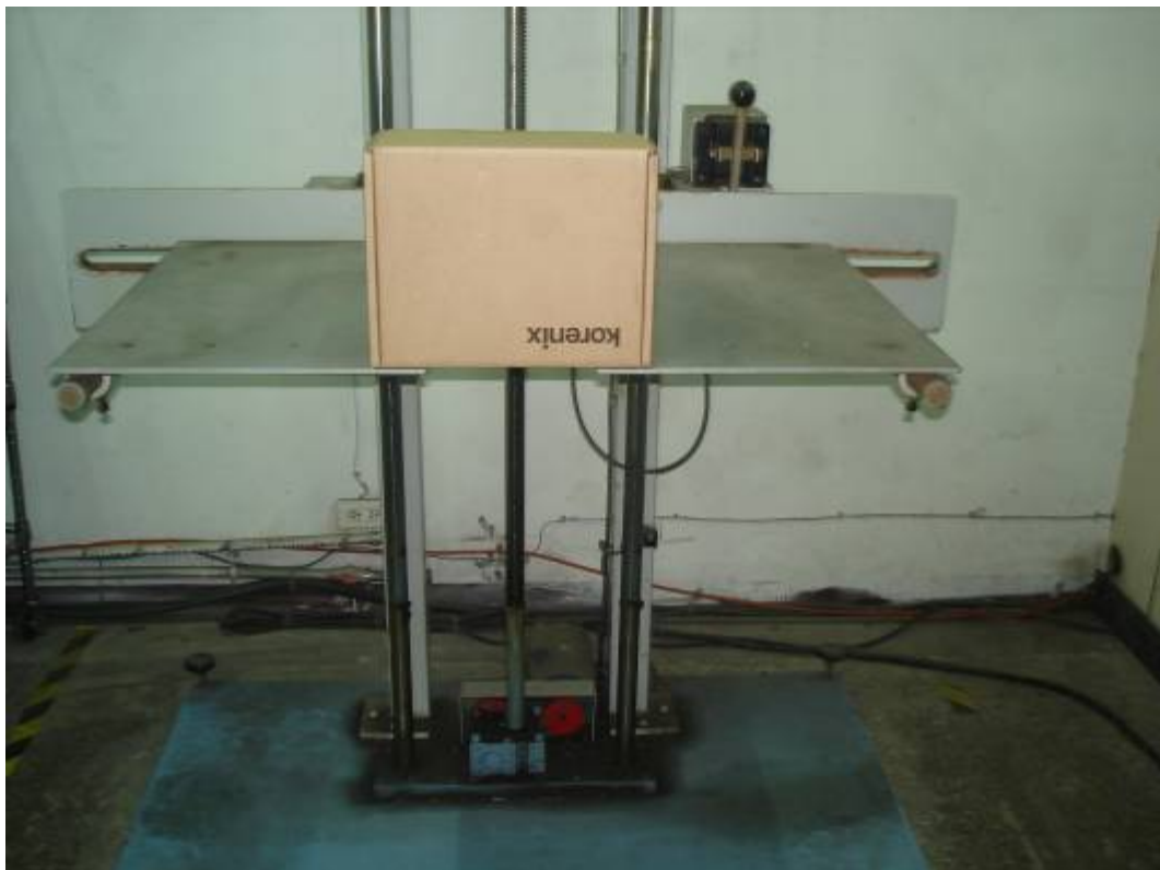
Fig. 14: Switching Hub (JetNet 5012G) Fall Test (Rear)
