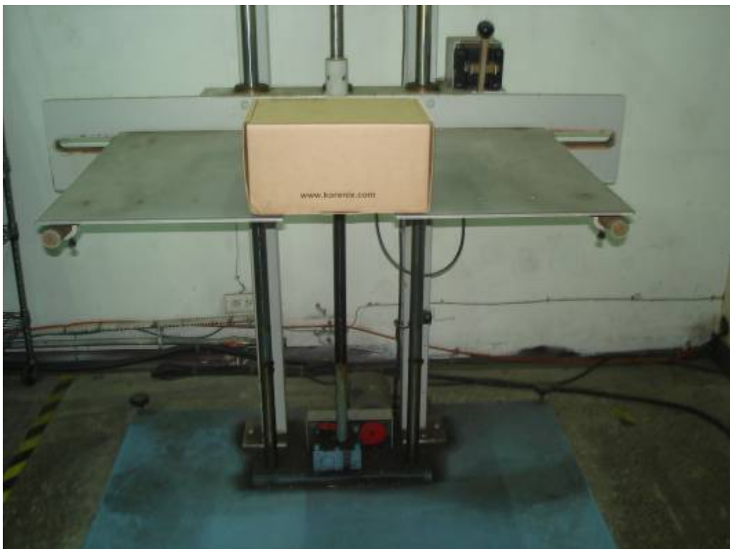
Fig. 18: Switching Hub (JetNet 5012G) Fall Test (Bottom)
