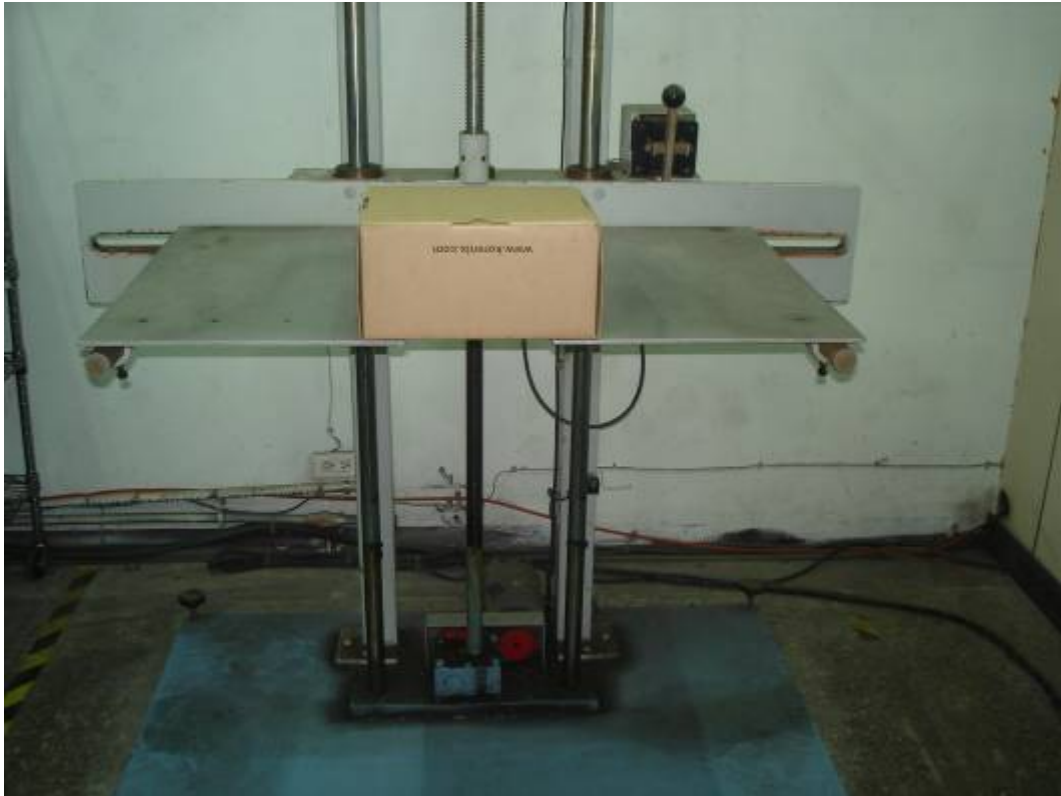
Fig. 17: Switching Hub (JetNet 5012G) Fall Test (Top)
