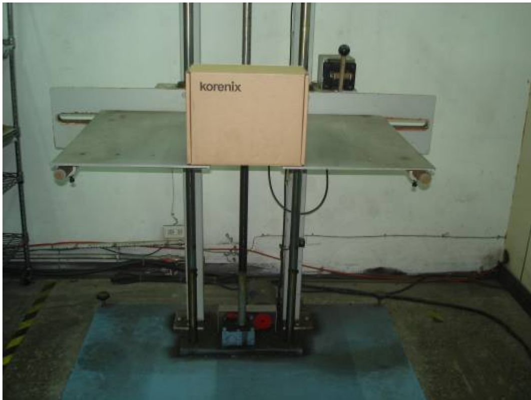
Fig. 13: Switching Hub (JetNet 5012G) Fall Test (Front)
