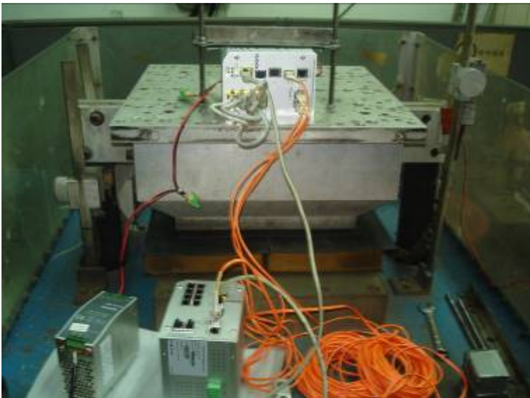
Fig. 8: Switching Hub (JetNet 5012G) Shock Test in \pm Y Axis -2
