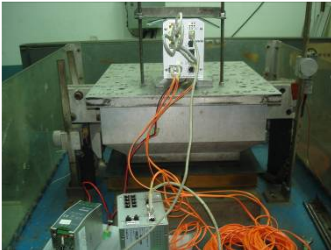
Fig. 9: Switching Hub (JetNet 5012G) Shock Test in \pm Z Axis -1
