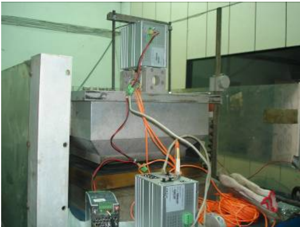
Fig. 7: Switching Hub (JetNet 5012G) Shock Test in \pm X Axis -2
