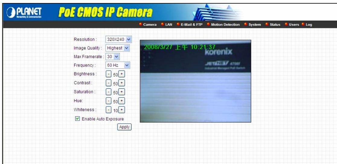
Note: Before you go to customer site, please setup the IP address for 4706 and IP camera. Korenix suggest you setup the new IP address for them in the same subnet. Thus you can easily exchange the display screen of the 4706 and IP camera.
