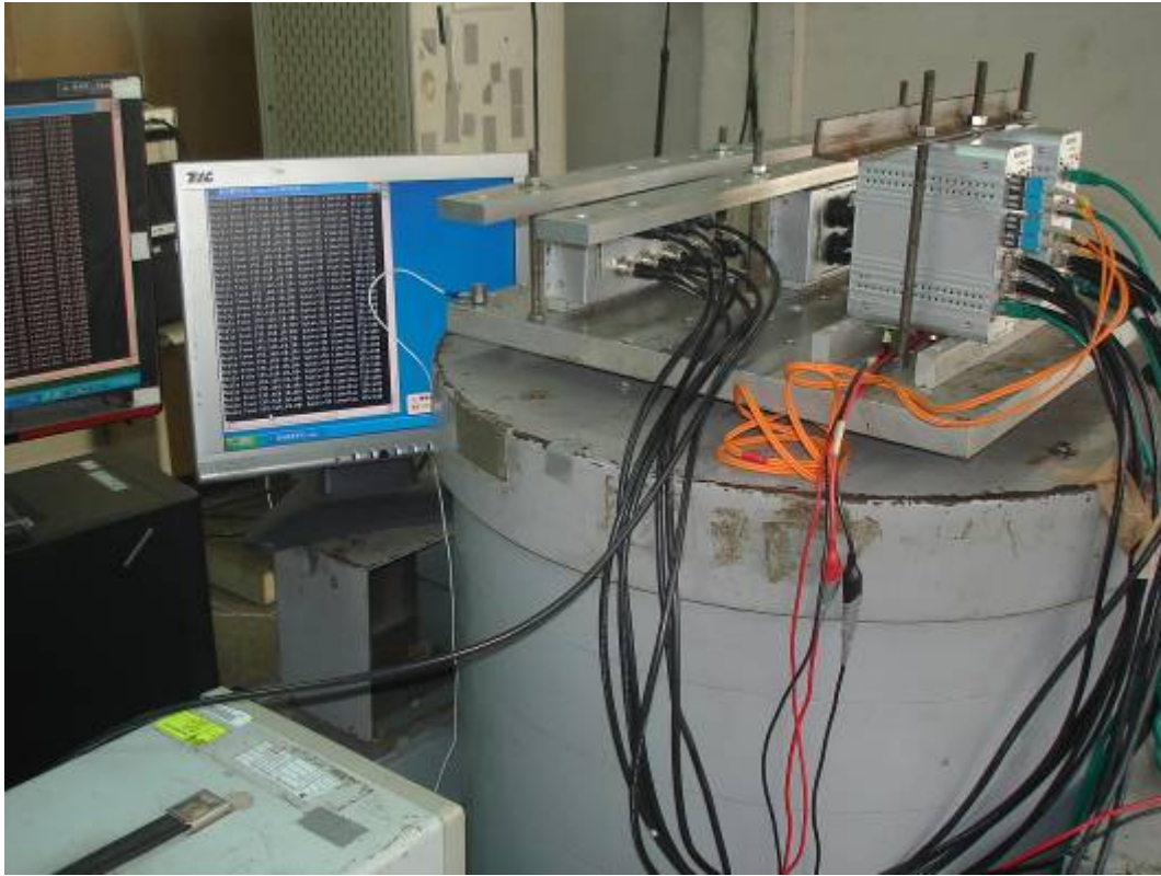
Fig. 3: Vibration Test in Z-Axis
