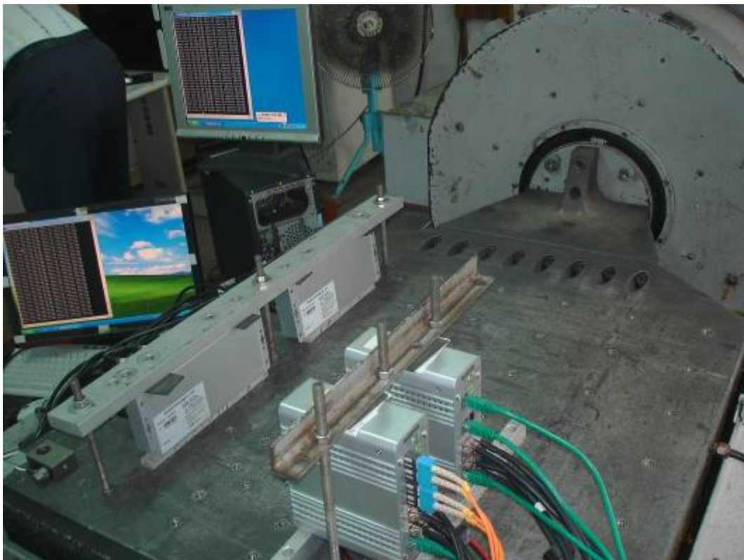
Fig. 2: Vibration Test in Y-Axis
