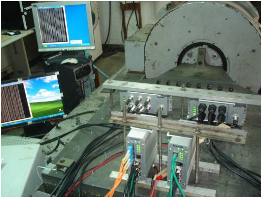
Fig. 1: Increased Vibration test in X-Axis
