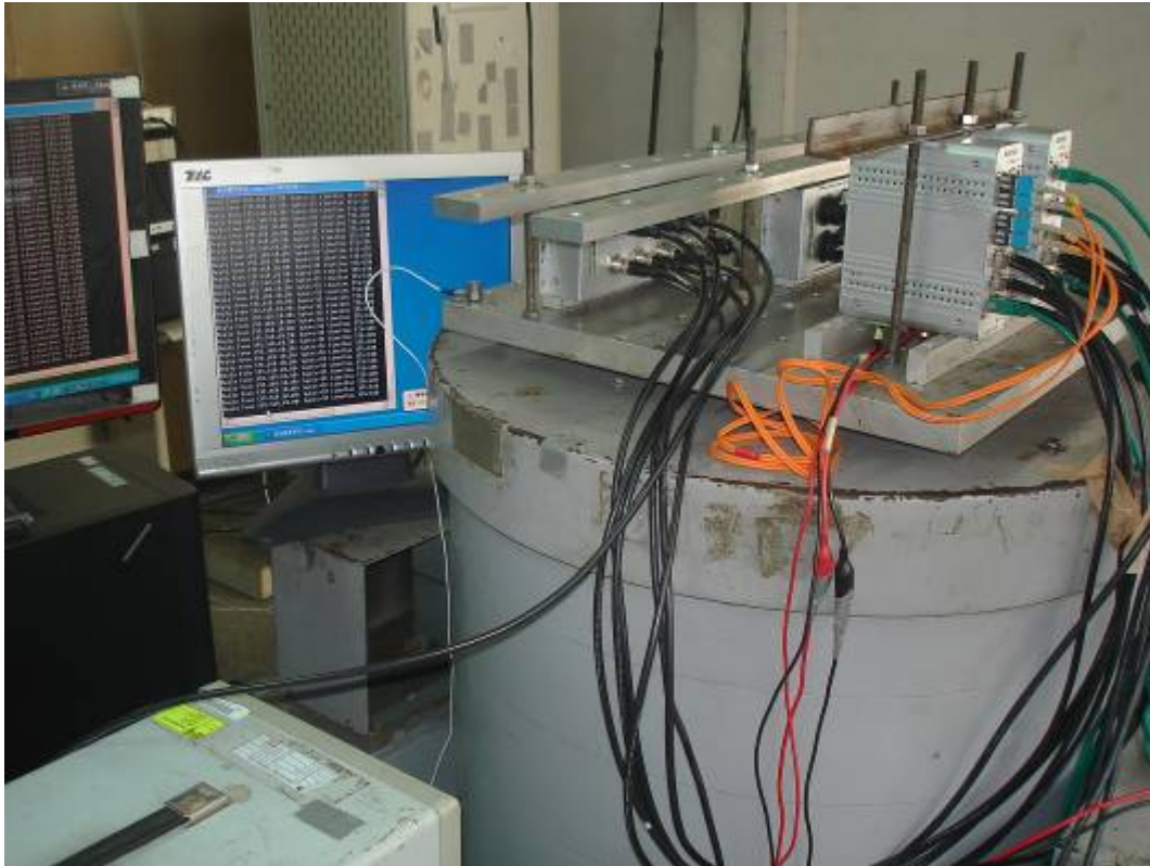
Fig. 3: Increased Vibration test in Z-Axis
