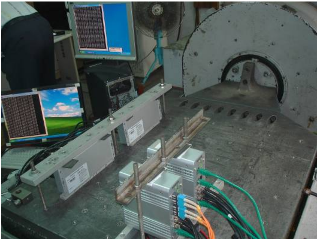
Fig. 2: Increased Vibration test in Y-Axis
